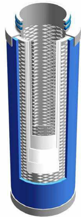
Cross section of the Ultrair depth filter
